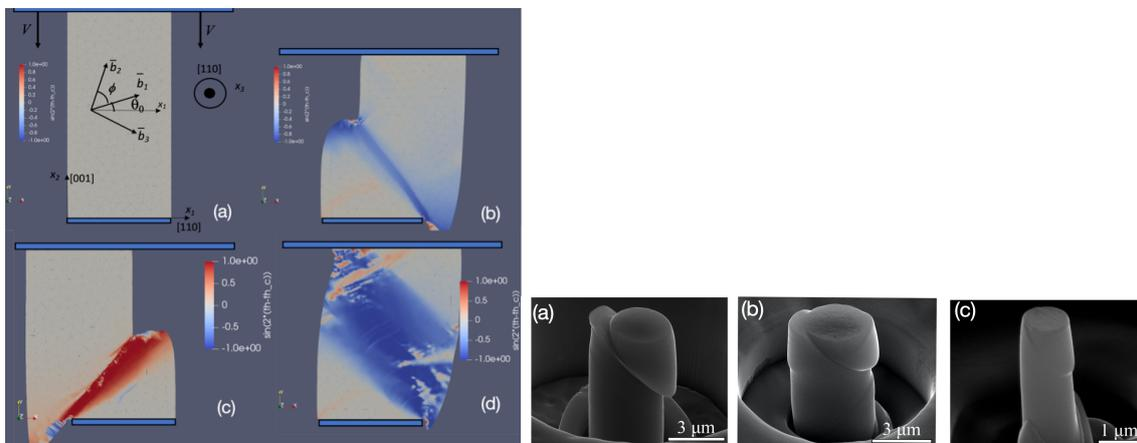
Left : Compression of a 2D nano-pillar using Eulerian plasticity approach (Free-Fem++ computations) for three different initial orientation of the crystal with the orientation misfit in color scale (from [4]). Right : Scanning electron microscopy images showing the deformed states pillars (experiments from [3])
